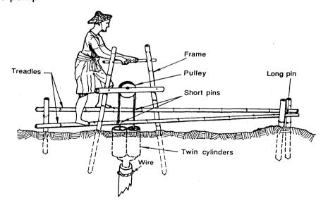
Figure 7: Treadle pump
