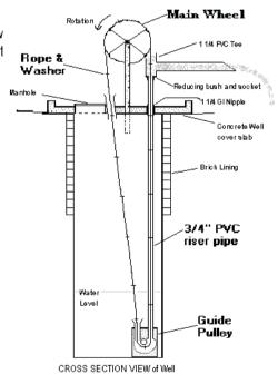
Figure 9: Rope and washer pump.
