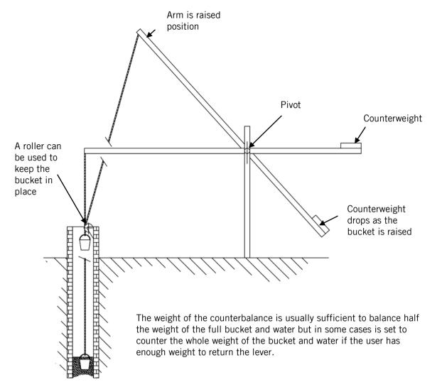
Figure 3: A counterpoise lifting device, also known as a shadouf, over an open well. A counterbalance helps lift the bucket of water.
