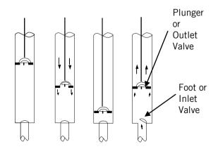
Figure 4: How most types of pump cylinders work.
